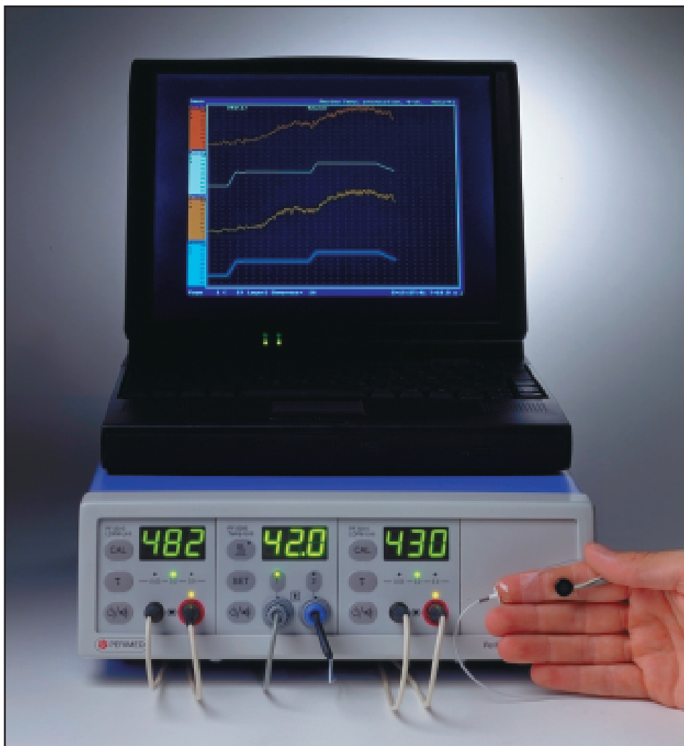
PeriFlux System 5000 equipped with 2 laser Doppler units, 1 temp unit, 1 small angled thermostatic laser Doppler probe, 1 skin temperature sensor and 1 probe for miniholders.
